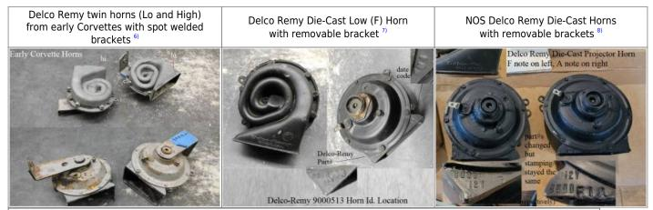
NOS Delco Remy D1935 F note and D1936 A note horns with the nut/screw on rear for brackets <sup>9)</sup>
