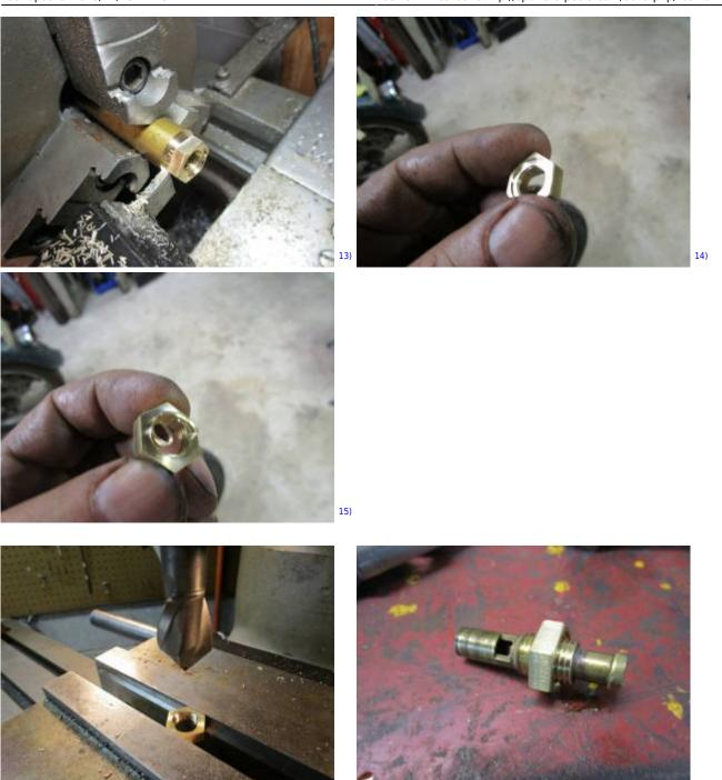
You end up with a needle seat position (read as float level) that can be adjusted on the side of the road in seconds.
