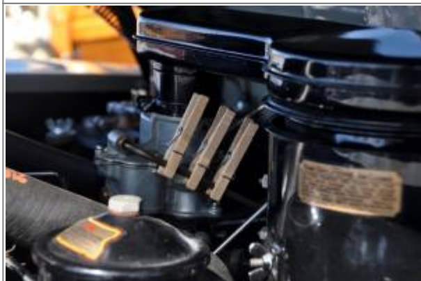
Clothes pins attached to fuel line for separation. 188)
