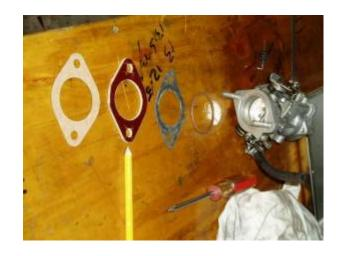
The Phenolic fiber spacer helps with hot idle or starting problems. One infuriatingly simple thing that affects idle, starting and carb farts when your engine is hot, is this phenolic fiber spacer. <sup>192)</sup> It's between the carb and manifold, which some models had and others did not. It stops engine heat from flowing into
