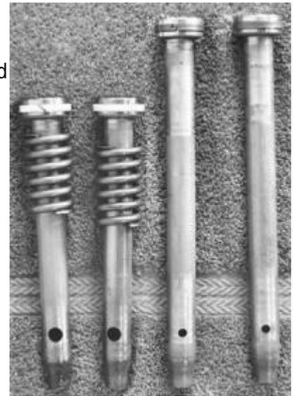
The length of the tube partly determines the overall slide movement range. The size of the holes at the bottom of the tube determines the rate of exchange of the oil between internal chambers when the fork is compressed. This helps control how quickly the forks compress.
