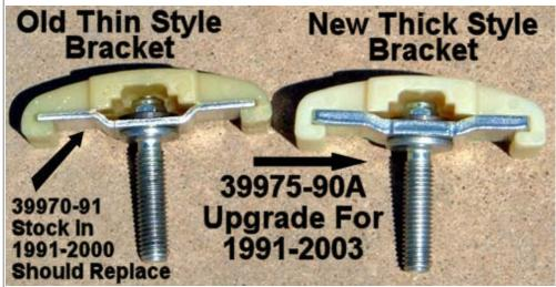
Upgrade 39975-90A should be used in place of 1991-2000 stock Chain Tensioner.
