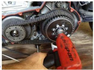
Normally when loosening or tightening these nuts, you will need to lock the hub & sprocket - Do not
