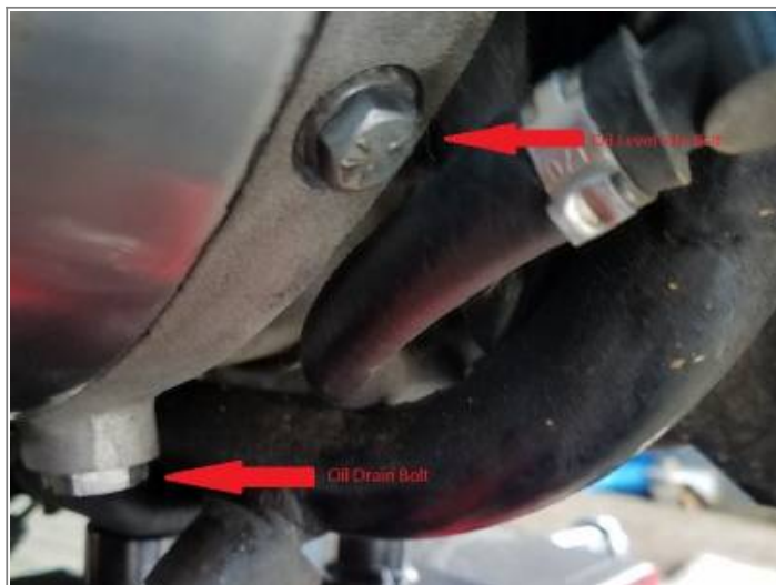
Primary / Transmission oil drain plug on 2001 Sportster 5)
