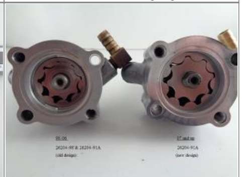
98 and 07 scavenger gerotors installed 15)
