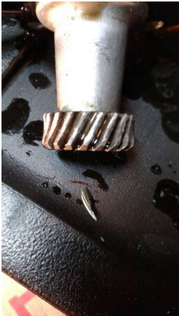
A chunk of a tooth from the oil pump gear fell out of the oil
