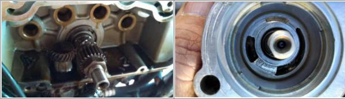
More oil pump and drive gear damage 56)
