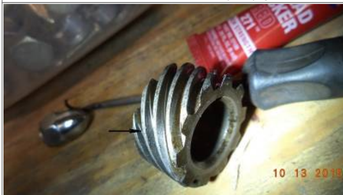
Teeth worn thin on the stock oil pump gear. 52)
