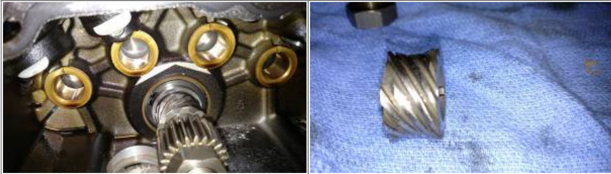
More oil pump and drive gear damage 56)
