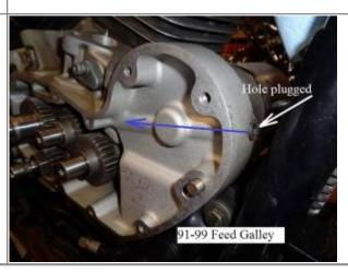
On 2000 and up engines, the oil feed galley is external. Oil travels to each lifter individually from this cavity. 5)
