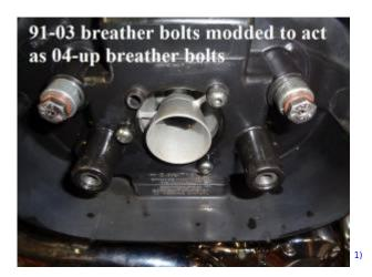
The internal hole on the outside end of 91-03 breather bolts is factory tapped 5/16"x24. It's not known at this time why as the thread are not used on OEM Sportsters.
