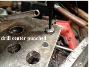
The small hole in 04-up breather bolts is 1/16" in diameter. However, as a test, 1/8" holes were drilled in these.
