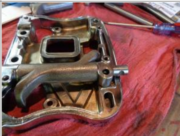
Aligning rocker arm shaft. 3)
