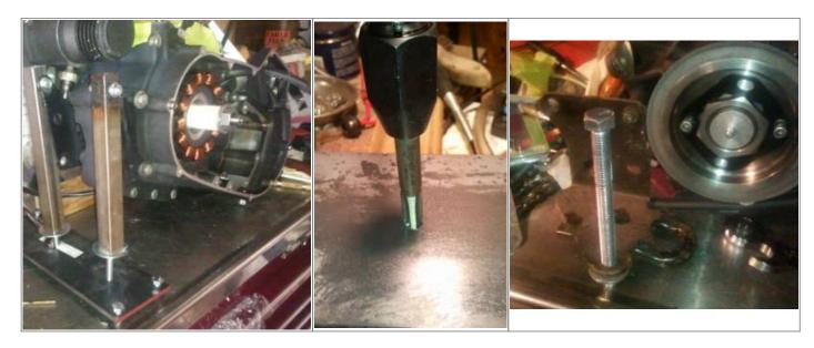
With the cylinder in place on the case, a construction type level was placed on top to insure it was level before drilling.
