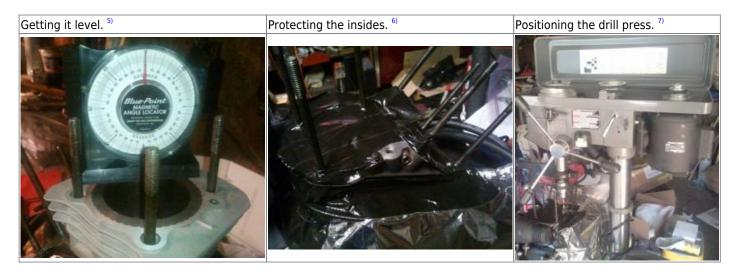
A 19/64" drill bit (which just barely fit inside the existing hole) was used to ensure the drill press was aligned to the hole.
