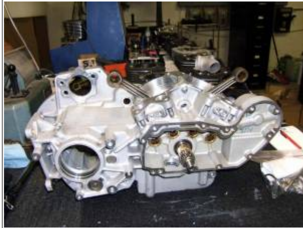
This picture shows proper alignment of the cam marks. Be sure you have the mark that's pointed to by the arrow. If it's not there, double check to make sure you haven't swapped the number 1 and 4 cams by mistake.
