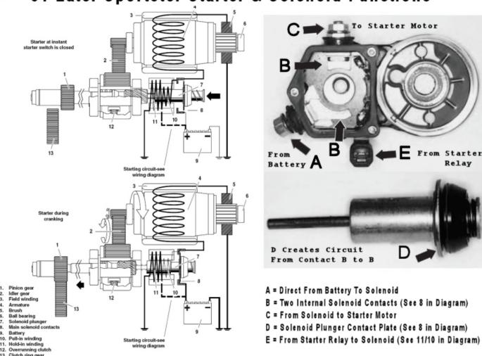
Technical Note - The pull-in windings are needed to initially move the plunger. Both the pull-in and hold-in windings are activated when the starter relay activates the solenoid. The power to the pull-in windings completes its path to ground thru the motor windings, while the hold-in windings have their own permanent ground path. Once the plunger moves forward into position, and the high-amperage contacts
