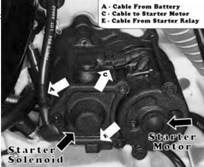
**Read and follow all the precautions listed above** for 'Testing the Starter Assembly while off the bike' to safely remove the starter from the bike. Once the starter/solenoid is safely off the bike and on the bench, you can proceed to test the solenoid windings.
