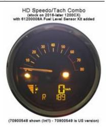
On the 2016-later 1200CX Roadster, the stock speedometer is P/N 70900549. It has a fuel level gauge that is not implemented with the stock low fuel sensor. However, testing by b0fh on the XLForum <sup>11)</sup> demonstrated that installing the 61200008A Fuel Level Sensor kit with this speedometer will indeed activate the fuel level gauge. (See the REF electrical section on speedometers)
